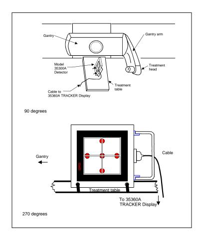
Figure 2-5. Setup for 90- and 270-Degree Angles (NOTE: Build-up not shown for clarity)
